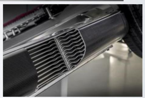
Hollow CFRP side sills contain aluminum fins (left) that channel cooling air from the front crush-can structures (twin projections at far right) to cool the batteries. SOURCE:WEA and The Engineer.co.uk
