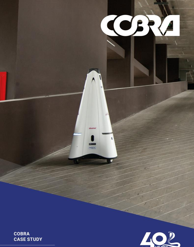
Composite Body Shell Cladding for Security Robots
