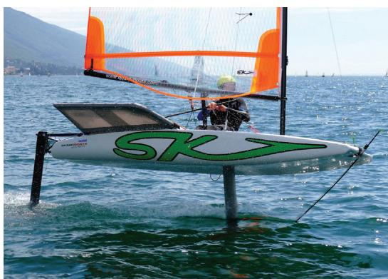
the water and skip back up again.' A further benefit is the ability for sailors to easily adjust their ride height on the fly, partially retracting the wand to reduce their elevation and stay in control in very strong or gusty winds.
