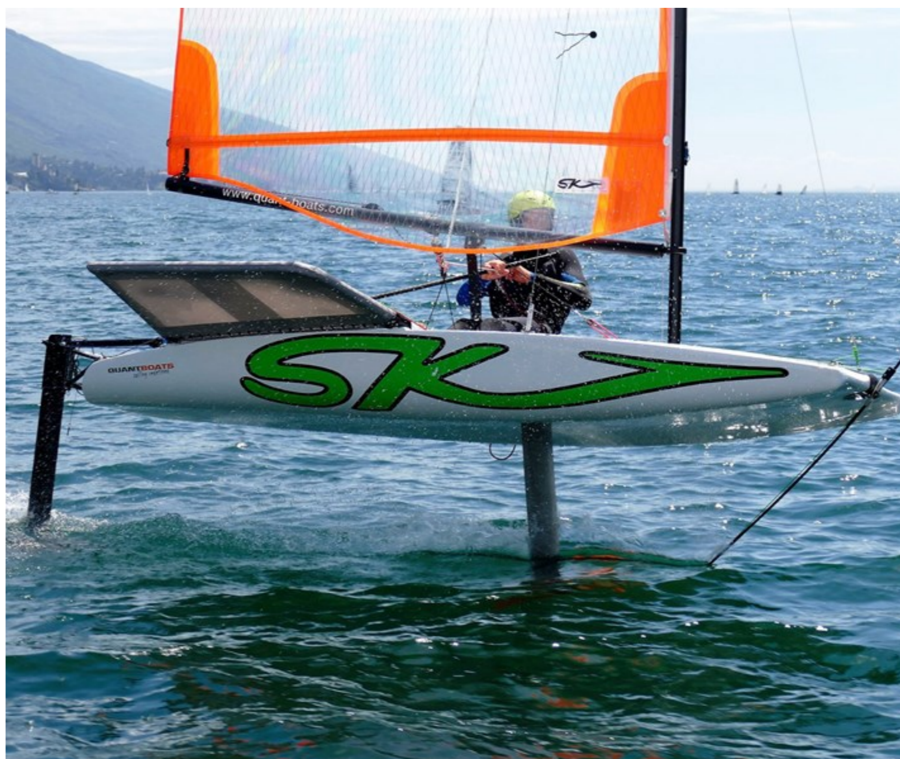
COBRA manufactures the 3.66m Skeeta hull using a molded EPS foam core blank, assembled with a mixture of woven and biaxial glass fibre fabrics, localized carbon fibre reinforcements and G-10 inserts. Source | COBRA International
