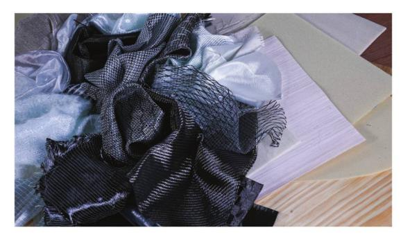
Over the past 25 years, Cobra has worked with the world's leading carbon fiber fabric producers, creating innovative alternatives when the traditional 3K fiber was unavailable, and focusing on spreading fibres into thinner plies to produce lighter and lighter biaxials. These lightweight (100-150gsm) cloths available today, were simply not possible 20 years ago, and many of these textiles saw their first real world applications at Cobra.
